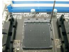
STEP 1: Lift Up The Socket Lever
